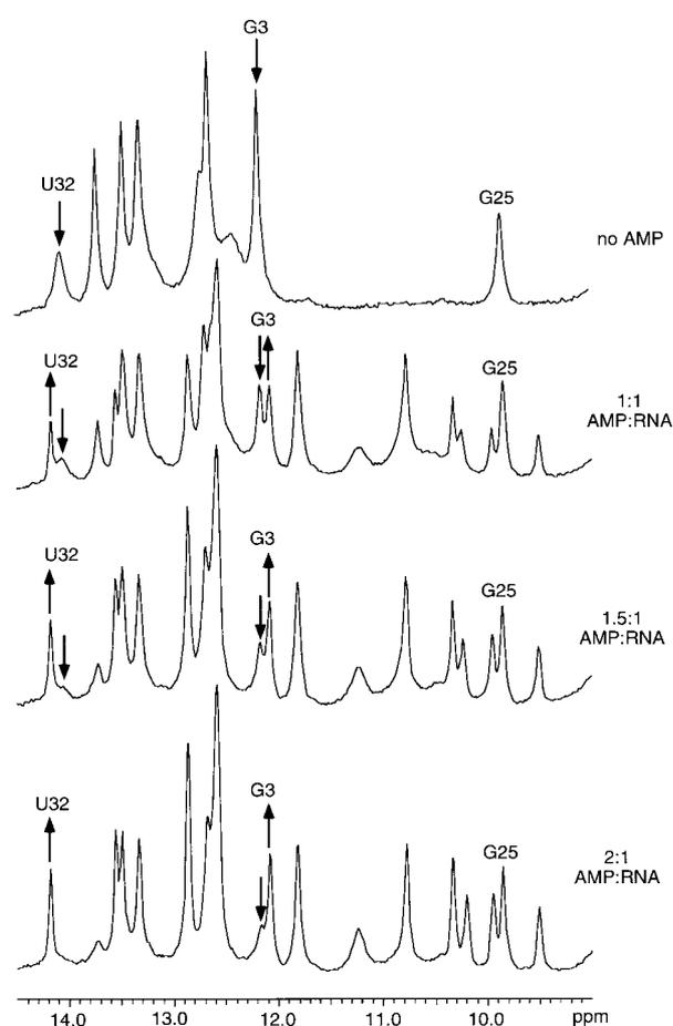
**Figure 3.** One-dimensional  $^1\text{H}$ NMR spectra of the exchangeable resonances of the G8A mutant aptamer at different AMP:RNA ratios. The spectra were measured at 274 K on a sample containing 0.8 mM RNA in 100 mM NaCl (pH 6.0). For each spectrum 128 scans of 4,096 complex points were acquired. The FIDs were zero-filled to 16 K and transformed after multiplication with an exponential function (LB = 15).
