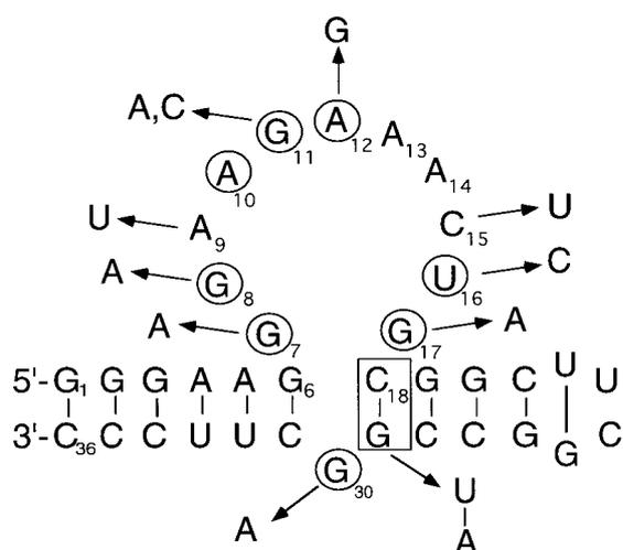
**Figure 1.** Sequence and secondary structure of the ATP-binding RNA aptamer. Base substitutions used in this study are labeled next to the original (wild-type) nucleotides. Nucleotides that were conserved in all the clones are circled.
