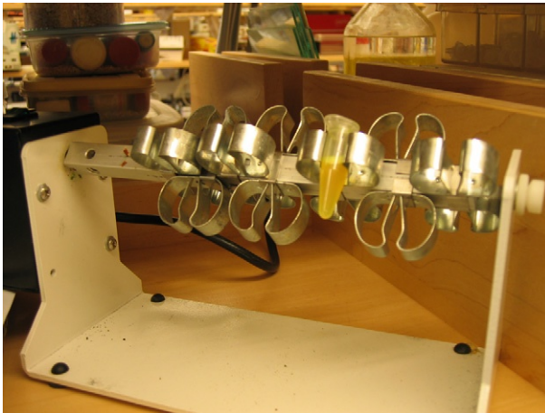
Figure 20.6 Vesicle suspension in a 1.5-ml microcentrifuge tube, on a bench top rotary tumbler.
