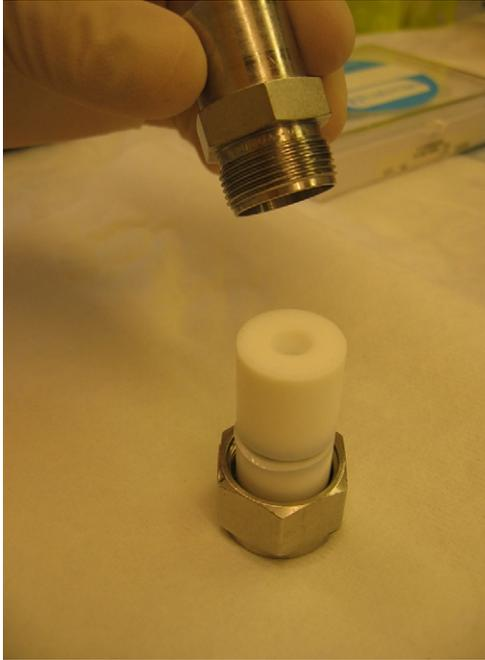
**Figure 21.4** Assembly of the internal membrane support parts with filter support and polycarbonate track-etched membrane in the middle.
