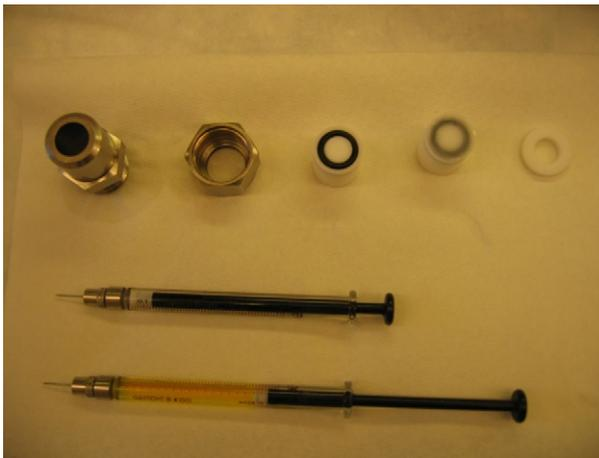
Figure 21.2 Hand-held mini-extruder with two gas-tight syringes.
